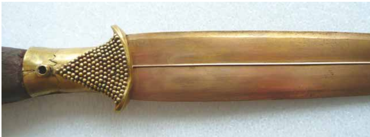
Figure 3. Dagger # 30-12-550, PG 1054. The dagger is composed of several types of gold. For the decoration of the hilt, greenish-yellow gold was used to manufacture some 400 nails, the collar and the sheets (left). The blade consists of a gold-silver alloy high in copper, gilded by a depletion gilding process. The golden surface is only in parts preserved (right). Length of the dagger: 33 cm. A similar feature is to be observe on the blade of a dagger from the Baghdad-Museum (Internet: www.baghdad-museum.org ).
