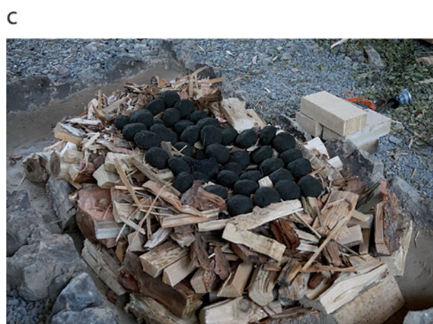
Figure 4. Roasting of the manure pellets, a) sketch of the roasting pile; b) temperature curve; c) roasting pile before fire is set; d) burned down roasting pile (modified after Rose, Hanning and Klein, 2019).
