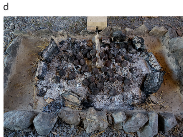
Figure 4. Roasting of the manure pellets, a) sketch of the roasting pile; b) temperature curve; c) roasting pile before fire is set; d) burned down roasting pile (modified after Rose, Hanning and Klein, 2019).
