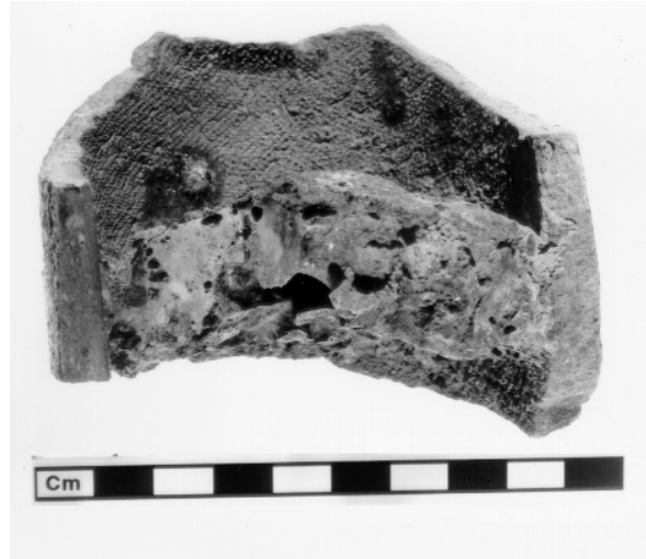
Fig. 6: Cross section through a typical slag cake as preserved regularly in the upper third of most crucibles. Note the high porosity of this slag.
